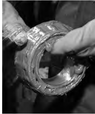
Fig. 23. Grease can easily be packed by hand.
